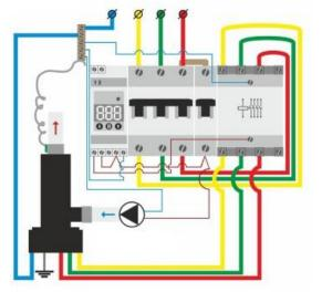
3) This is the classic connection diagram for three-phase electrode boilers. Such as: Geyser 9, Geyser 15 and Wulkan 25
