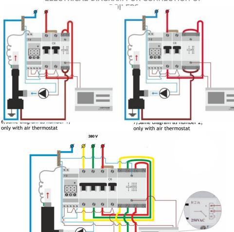
8) This is a wiring diagram showing how to connect an air thermoregulator (same diagram as number 3) to an existing control unit with a TR-16 temperature controller installed. For example, there is a Computherm g7, but any air temperature controller can be used.
