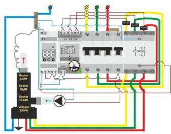
5) An ammeter has been added to this diagram. For three-phase boilers: Geyser 6, Geyser 9 Geyser 15 and Volcano 25.
