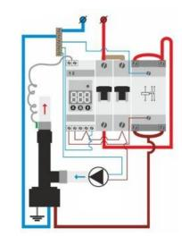
1) This is a simple wiring diagram for single phase boilers up to 3 kW.
